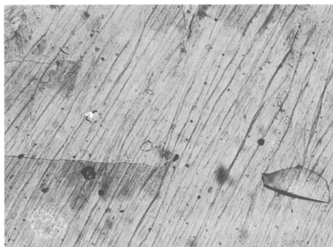
Figure 5 Microstructure of benzidine- \alpha -naphthol addition compound, \times 100 .
