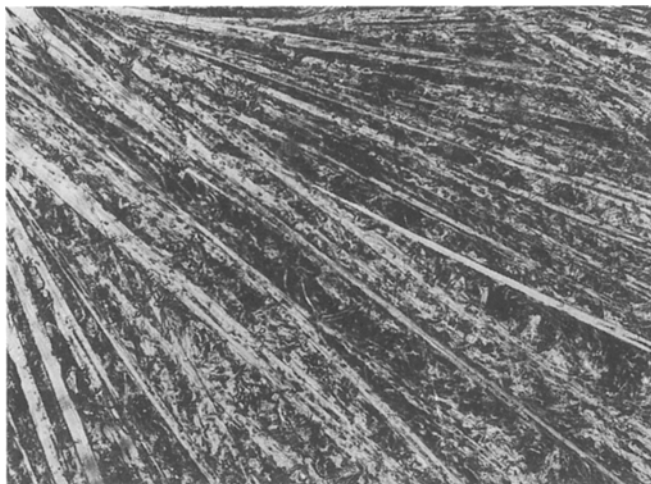
Figure 4 Microstructure of benzidine- \alpha -naphthol eutectic, E 2 , \times 100 .
